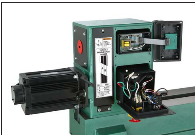
Figure 58. Control panel wiring.
